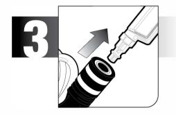
Attach Tire Inflation Gun to the coil hose from the compressor
