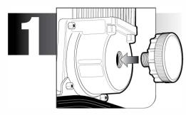
Make sure the intake air filter is installed where the red plug was removed from the intake on the compressor.
