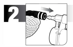
Attach the primary coil hose to the quick connect coupler on the compressor. If needed, attach the extension coil hose to the primary hose.
