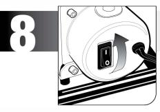
Turn the compressor on (I for On, 0 for Off). The compressor will fill up the coil hose(s) with air pressure and then shut itself off, this is normal.
