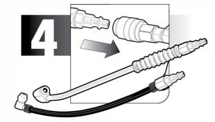
Attach either the 90 degree twist on chuck, or the 45 degree chuck to the quick connect coupler on the end of the Tire Inflation Gun.
