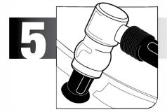
Attach the other end of the 45 degree chuck or the 90 degree chuck to the valve stem on your tire.
