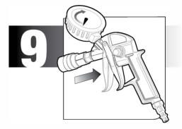
Pull the trigger on the inflation gun to allow air to flow into the tire, at this time the compressor will turn itself back on and begin filling the tire.
