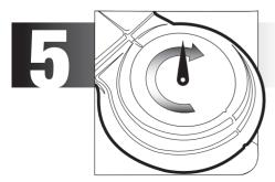
To check tire pressure, manually turn the compressor off. Once the gauge settles, that will be the accurate pressure in the tire.
