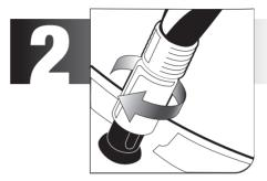
Attach the end of the air hose to the valve stem on your tire
